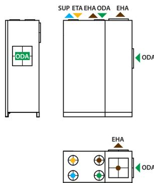
▶ ODA – outdoor intake      ▶ SUP – supply air      ▶ ETA – extract indoor      ▶ EHA – exhaust air
